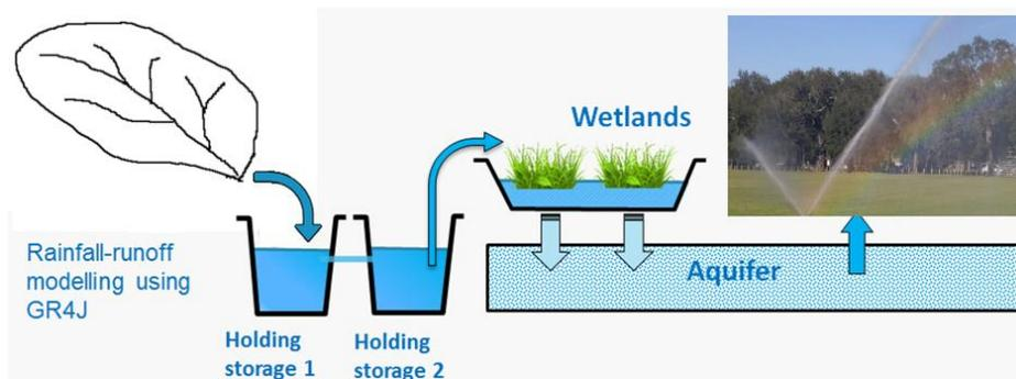
Schematic of the Parafield Managed Aquifer Recharge system.
